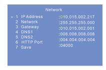
IP address: Select IP address and press "ENTER" to set the IP address. The default IP address is DHCP.
