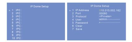
Press "SHIFT" to switch the PTZ camera listed in the IP dome setup interface in sequence.
