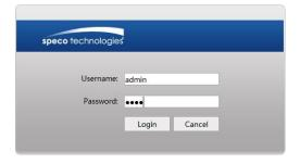
The login interface is shown above. Default username is **admin** and password is **1234**. After logging in, follow directions to install applicable plug-ins for viewing video if prompted.
