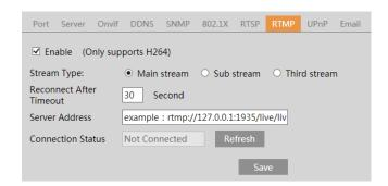
Check "Enable", select stream type, set the reconnection time after timeout and server address as needed. Server address: Enter the server address allocated by the third party server.
