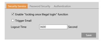
In order to prevent against malicious password unlocking, "Locking once illegal login" function can be enabled here. If this function is enabled, login failure after trying five times will make the login interface locked. The camera can be logged in again after a half hour or after the camera reboots.
