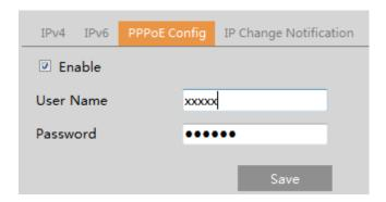
Either of these two network connection methods can be used. If PPPoE is used to connect internet, the camera will get a dynamic WAN IP address. This IP address will change frequently. To be notified, the IP change notification function can be used. Click "IP Change Notification Config" to go to the interface as shown below.
