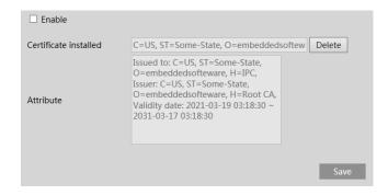
There is a certificate installed by default as shown above. Enable this function and save it. Then the camera can be accessed by entering https://IP: https://IP:
