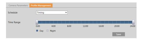
Drag "\bigcap" icons to set the time of day and night. Blue means daytime and blank means night time. If the current mode of camera parameters is set to "Timing", the image configuration mode will automatically switch between day and night according to the schedule.
