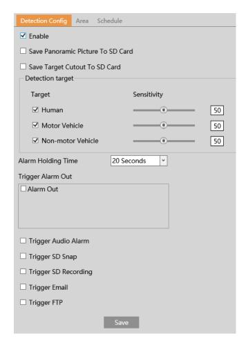
1. Enable line crossing alarm and select the snapshot type and the detection target.
