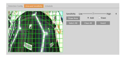
Move the "Sensitivity" scroll bar to set the sensitivity. A higher sensitivity value means that motion will be triggered more easily. Select "Add" and click "Draw". Drag the mouse to draw the motion detection area; Select "Erase" and drag the mouse to clear motion detection area.
