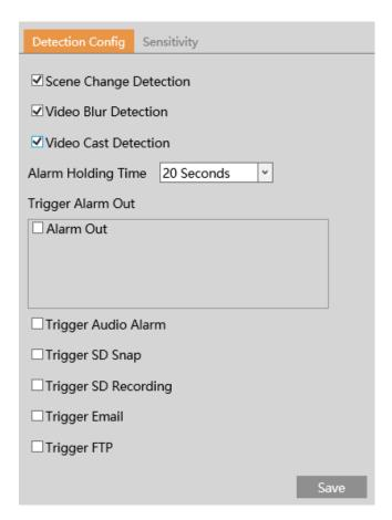
1. Enable the applicable detection that is desired.
