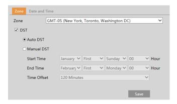
Select the applicable time zone and enable / disable DST as needed. Click the "Date and Time" tab to set the time, date and time format.
