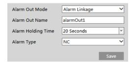
Alarm Out Mode: Alarm linkage, manual operation, day/night switch linkage, and schedule are optional.
