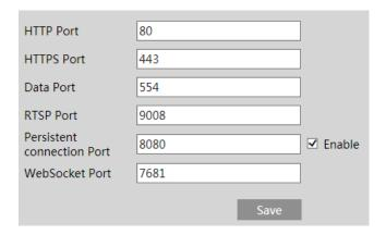
**HTTP Port**: The default HTTP port is 80. It can be changed to any port which is not occupied. **HTTPS Port**: The default HTTPs port is 443. It can be changed to any port which is not occupied.
