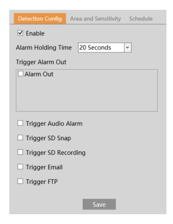
1. Check "Enable" check box to activate motion-based alarms. If unchecked, the camera will not send out any signals to trigger motion-based recording to the NVR or CMS, even if there is motion in the video.
