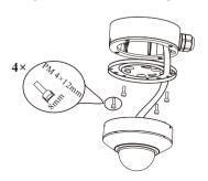
3. Align the three screw holes of the adapter with the screws of the mounting base.
