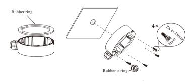
3. Use four screws provided to install the adapter to the junction box.
