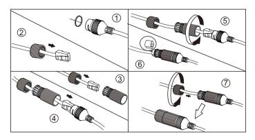
\* If the RJ 45 connector of the network cable has a jacket and cannot be threaded through the kit, remove the jacket. If the jacket cannot be removed, cut off the connector and install an RJ 45 connector without the jacket.
