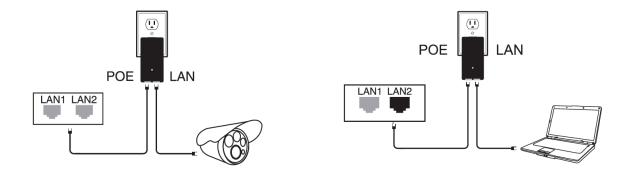
The bottom of the adapter has two RJ45 connections. One marked POE and one marked LAN.
