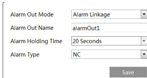
**Alarm Out Mode:** Alarm linkage, manual operation, day/night switch linkage and schedule are optional.
