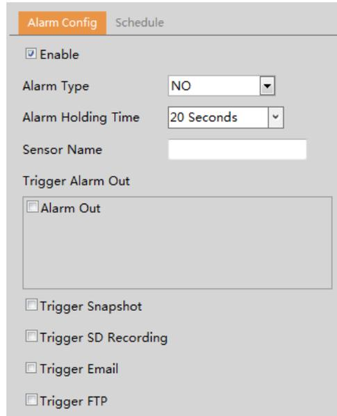
1. Click “Enable” and set the alarm type, alarm holding time and sensor name.
