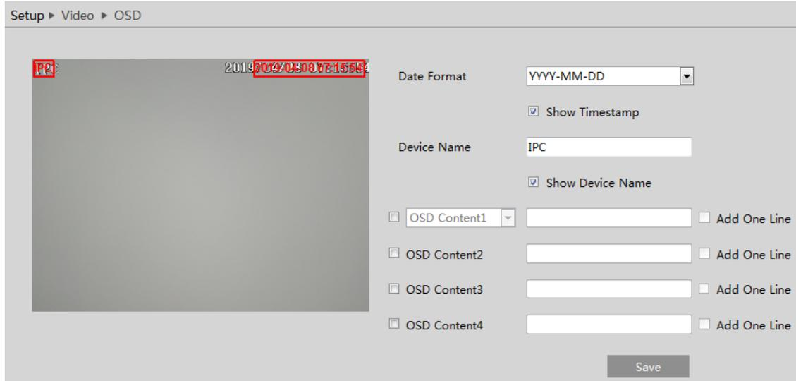
Set time stamp, device name, OSD content and picture overlap here. After enabling the corresponding display and entering the content, drag them to change their position. Then click the “Save” button to save the settings.
