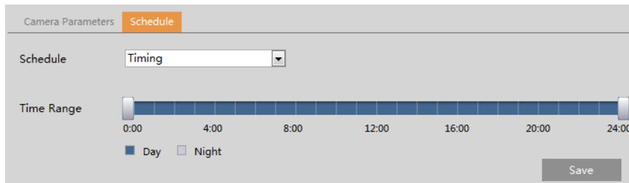
Drag “🕒” icons to set the time of day and night. Blue means day time and blank means night time. If the current mode of camera parameters is set to “Timing”, the image configuration mode will automatically switch between day and night according to the schedule.
