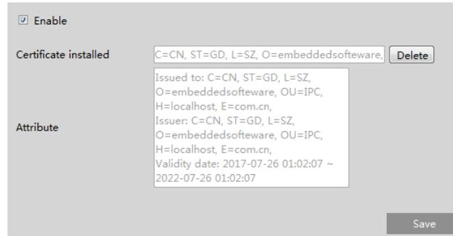
There is a certificate installed by default as shown above. Enable this function and save it. Then the camera can be accessed by entering https://IP: https port via the web browser (eg. https://192.168.226.201:443).
