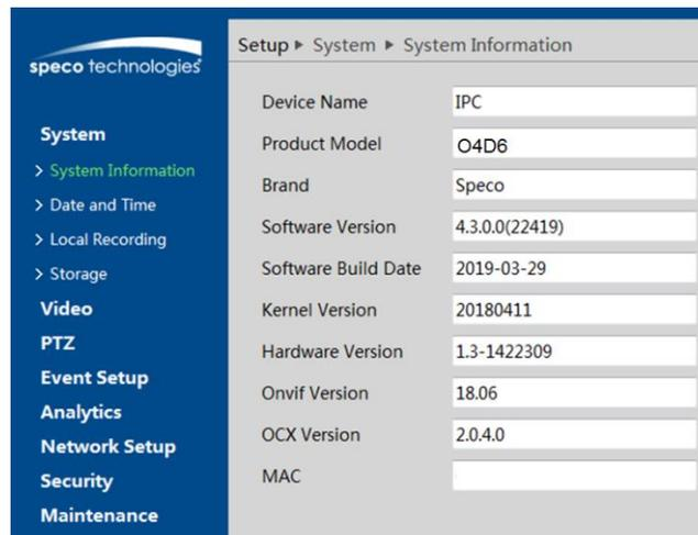
The screenshot shows the 'System Information' configuration page in the Speco Technologies interface. The breadcrumb path is 'Setup > System > System Information'. The left sidebar contains navigation options: System (selected), > System Information, > Date and Time, > Local Recording, > Storage, Video, PTZ, Event Setup, Analytics, Network Setup, Security, and Maintenance. The main content area lists the following system information:
