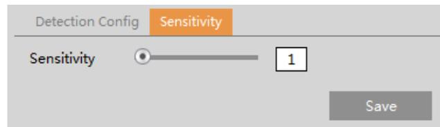
Drag the slider to set the sensitivity value or directly enter the sensitivity value in the textbox. Click "Save" button to save the settings.
