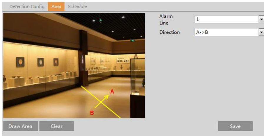
Set the alarm line number and direction. Up to 4 lines can be added. Multiple lines cannot be added simultaneously.
