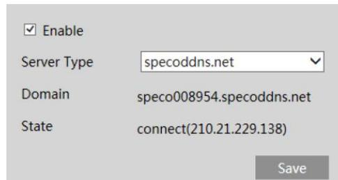
The screenshot shows the same DDNS configuration panel after being updated. The "Enable" checkbox is now checked. The "Server Type" remains "specoddns.net". The "Domain" field now contains "speco008954.specoddns.net". The "State" is now set to "connect(210.21.229.138)". The "Save" button is still present at the bottom right.
