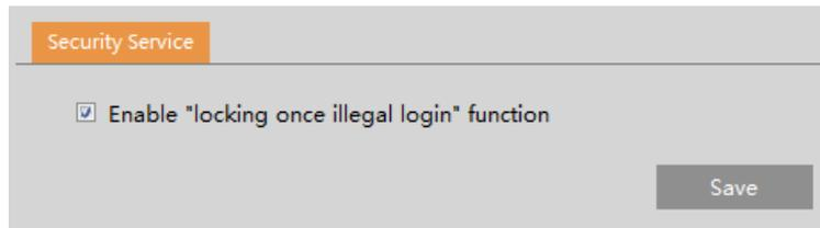
In order to prevent against malicious password unlocking, “locking once illegal login” function can be enabled here. If this function is enabled, login failure after trying six times will make the login interface locked. The camera can be logged in again after a half hour or after the camera reboots.
