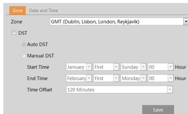
The screenshot shows the 'Date and Time' configuration page. The 'Zone' is set to 'GMT (Dublin, Lisbon, London, Reykjavik)'. The 'DST' checkbox is unchecked. Under 'DST', 'Auto DST' is selected. The 'Start Time' is set to 'January', 'First', 'Sunday', '00' Hour. The 'End Time' is set to 'February', 'First', 'Monday', '00' Hour. The 'Time Offset' is set to '120 Minutes'. A 'Save' button is located at the bottom right.
