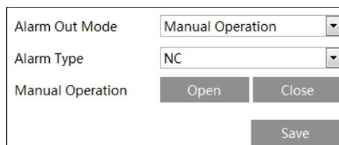
**Day/Night Switch Linkage:** Having selected this mode, select the alarm type and choose to open or close alarm out when the camera switches to day mode or night mode.
