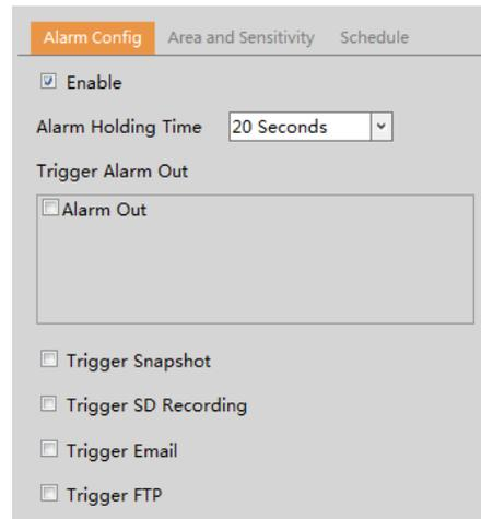
1. Check “Enable” check box to activate motion based alarms. If unchecked, the camera will not send out any signals to trigger motion-based recording to the NVR or CMS, even if there is motion in the video.
