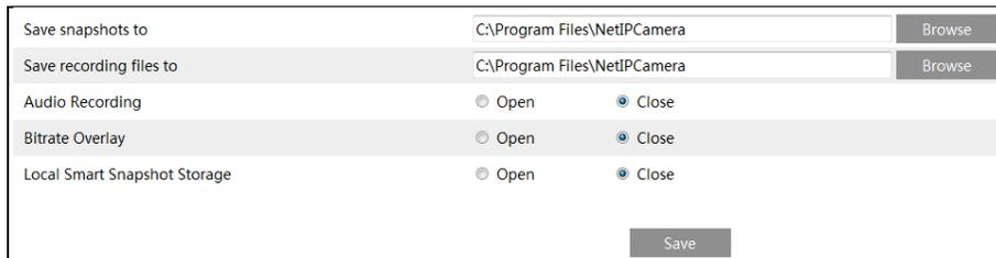
Additionally, the snapshots triggered by smart events (including face detection, line crossing detection and intrusion detection) can be selected to save to the local PC.
