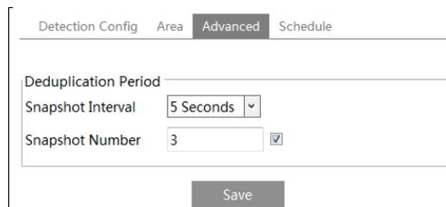
Snapshot Interval: If 5 seconds is selected, the camera will capture the same target once every 5 seconds during its continuous tracking period.
