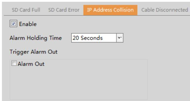
2. Click “Enable alarm” and set the alarm holding time.
