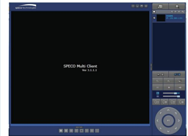
SpecoTech Multi-Client Viewer Software is a multiple site monitoring client software that allows streaming of video and audio, and transmission of alarm signals from the NVRs over the network. The SpecoTech Multi-Client can display up to 16 NVRs and supports dual monitors.
