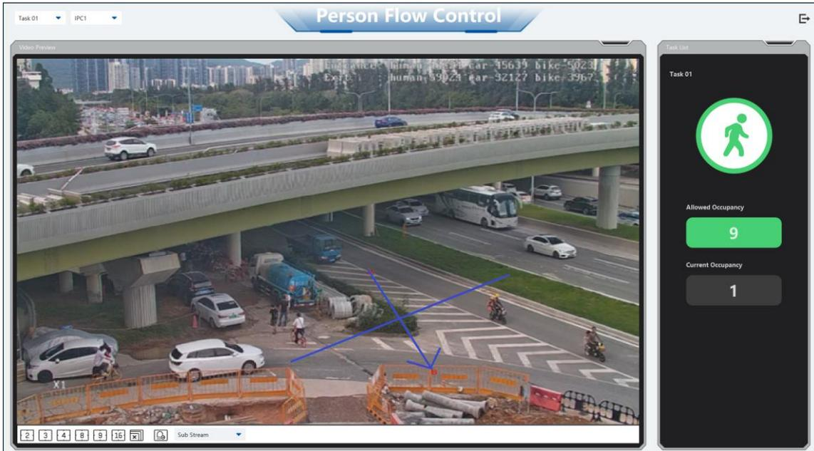
In the above interface, you can switch the camera and view the image. When the people/vehicles inside exceed the threshold, the icon will turn red.
