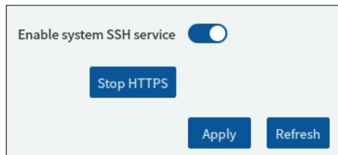
In this interface, you can enable system SSH service. This service is for test. In addition, you can also disable HTTPS here.
