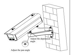
6. Adjust the depression angle and pan angle by loosening the two screws indicated above. After that, tighten these two screws
