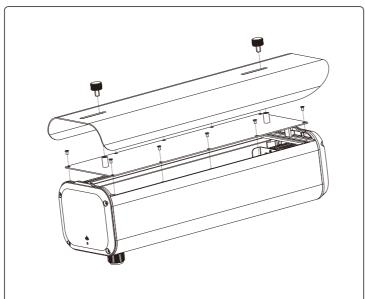
Unscrew the sunshield and then remove the upper cover of the housing as shown above.
