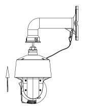
2. Secure the PTZ camera to the bracket with screws.
