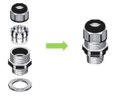
2. Put a network cable and grounding wire through the connector.
