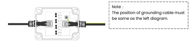
7. Put on the cover and screws to firmly fix the waterproof case.
