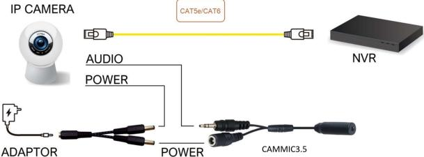
NOTE: Since the CAMMIC3.5 is a high-sensitivity microphone, it should be installed at least 15' away from any speakers to avoid audio reverberation.
